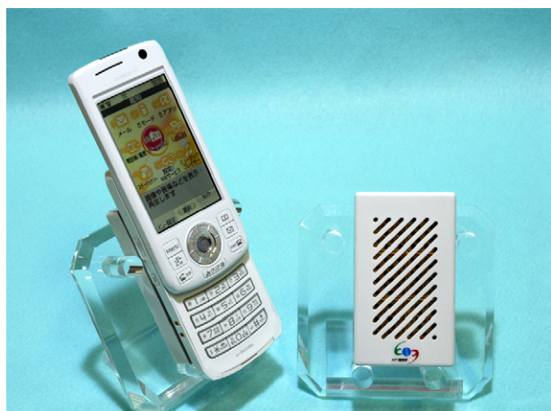
Fig. 15. Small PEMFC system (right) and the cell phone (left) is operated by the small PEMFC.
